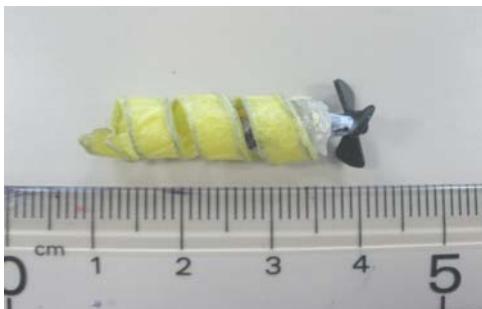
Figure 18 The prototype of the optimised head part (one magnet) (see online version for colours)
