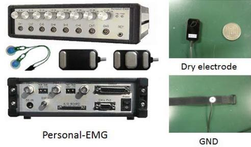
Figure 3. Experimental setup of sEMG acquisition
