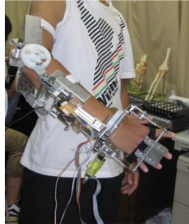
Figure 1. the Upper Limb Exoskeleton Rehabilitation Device (ULERD)
