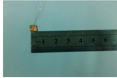
Fig. 7 The shape and size of the developed sensor
