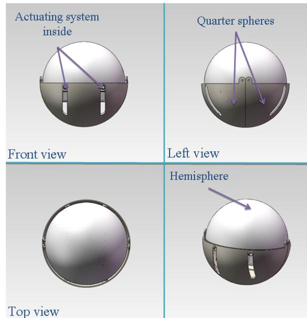
Fig. 3 Proposed mother robot (Closing state)
