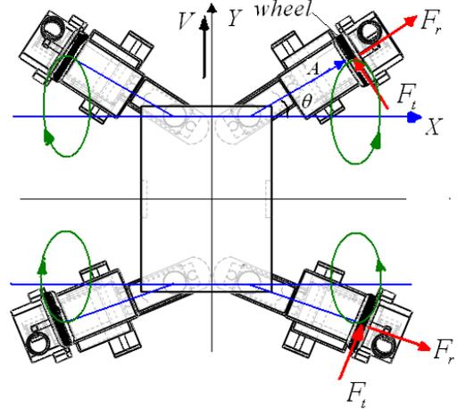
Fig. 10 Body coordinates and cyclic trajectory in straight motion
