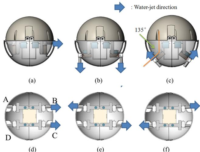
Fig. 5 Underwater motions. Front view: (a) Moving forward, (b) Surfacing, (c) Diving; Top view: (d) Moving forward, (e) Clockwise rotation, (f) Counter-clockwise rotation.
