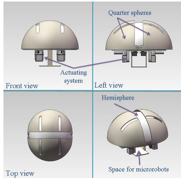
Fig. 2 Proposed mother robot (Opening state)
