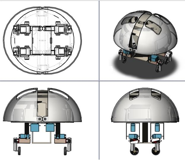
Fig. 8 Improved structure with four passive wheels
