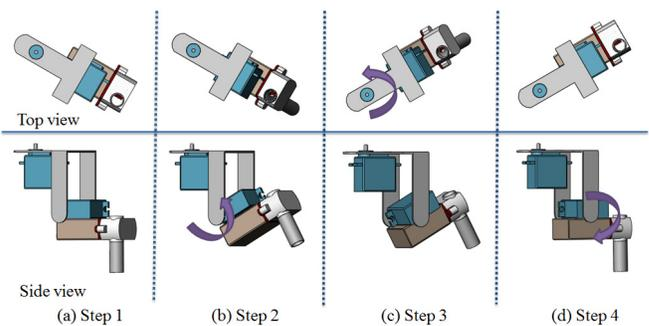
Fig. 4 Walking motion for one leg. (a) Lift up, (b) Swing forward, (c) Drop down, (d) Swing backward.
