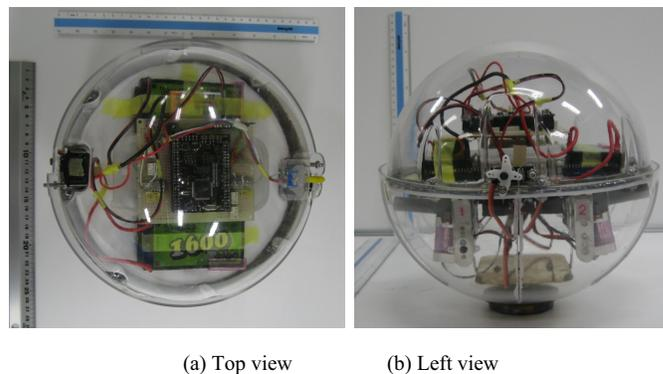
Fig. 6 Prototype spherical mother robot
