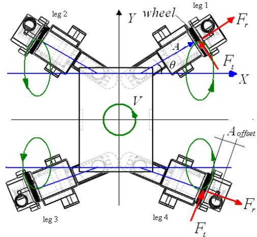
Fig. 11 Cyclic trajectory in angular motion
