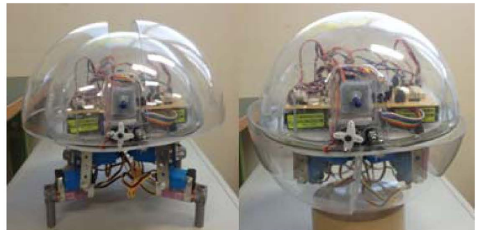
Fig. 4 The prototype spherical mother robot
