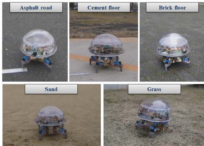
Fig. 5 Walking experiments in different terrains
