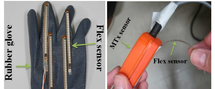
(a) Rubber glove with flex sensors (b) Flex sensor attached with MTx sensor
