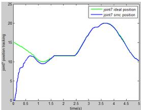
Fig.4 Position tracking of joint 7.
