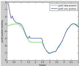
Fig.2 Position tracking of joint 5.
