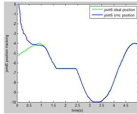
Fig.3 Position tracking of joint 6.
