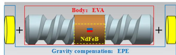
Figure 19. The gravity compensation of the microrobot
