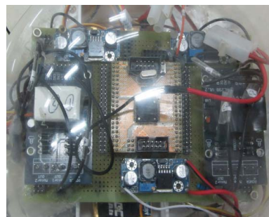
Fig. 4 Prototype of the control system
