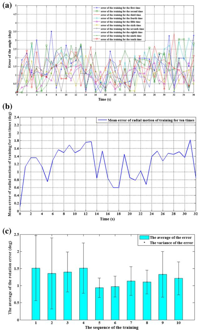
**Fig. 15** Experimental results of rotation experiment. **a** The radial error of 10 experiments. **b** The radial average error of 10 experiments. **c** The variance and the average of the rotation error
