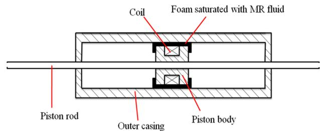
**Fig. 10** The conceptual diagram of MR fluid damper assembly
