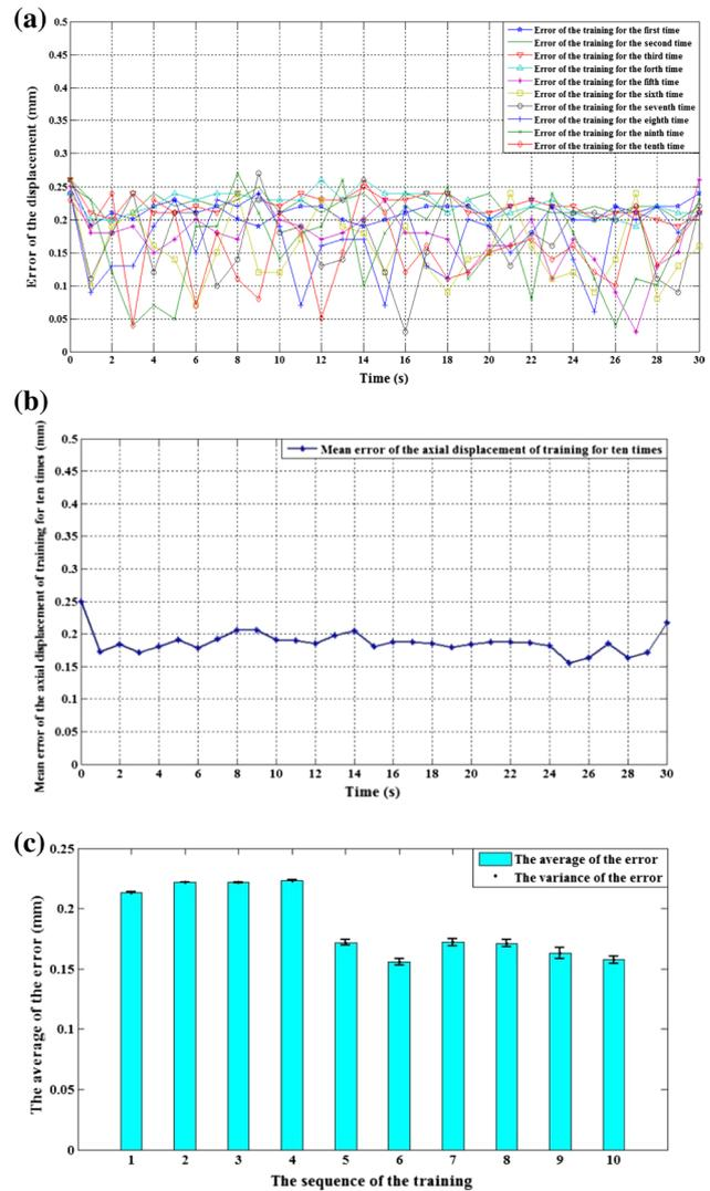
**Fig. 14** Experimental results of axial movement. **a** The axial error of 10 experiments. **b** The axial average error of 10 experiments. **c** The variance and the average of the displacement error
