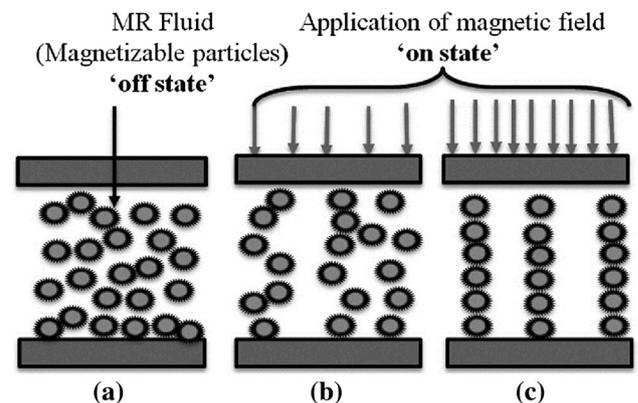
**Fig. 11** Chain structures of magnetorheological particles **a** magnetorheological fluids in 'off state,' **b, c** magnetorheological fluid in "on state" and the magnitude of magnetic field **(b)** is smaller than **(c)**
