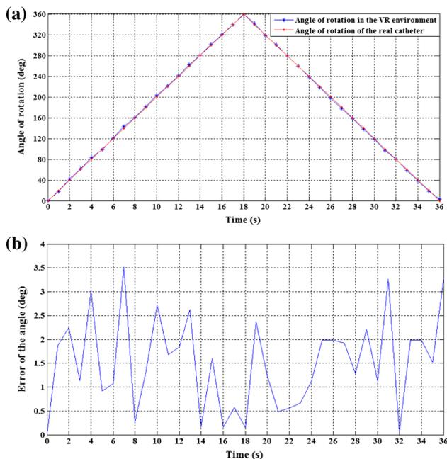
**Fig. 9** Experimental results of the radial rotation. **a** The rotation tracking curves between real catheter and catheter model. **b** Error analysis in VR environment
