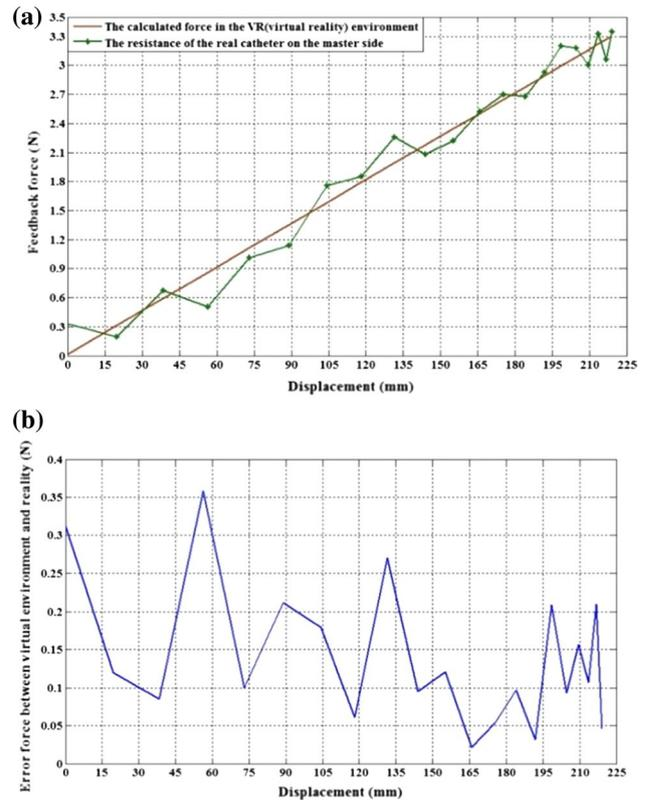
**Fig. 12** The experimental result of feedback force. **a** The force curves between catheter resistance and calculated force in VR. **b** Force error analysis
