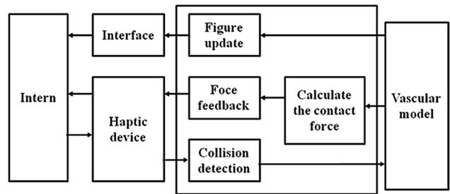
**Fig. 2** The Functional block diagram of the developed system
