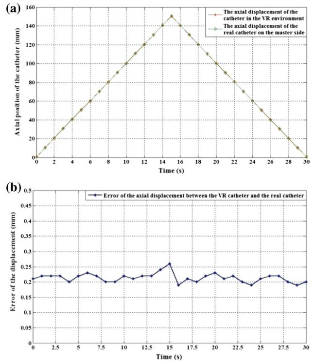
**Fig. 8** Experimental results of the axial insertion. **a** The axial movement curve of the real catheter and the catheter model. **b** Error analysis
