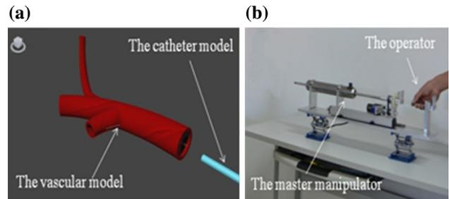
**Fig. 3** a The vascular and the catheter model. b The master manipulator. The developed master manipulator based on MRF damper
