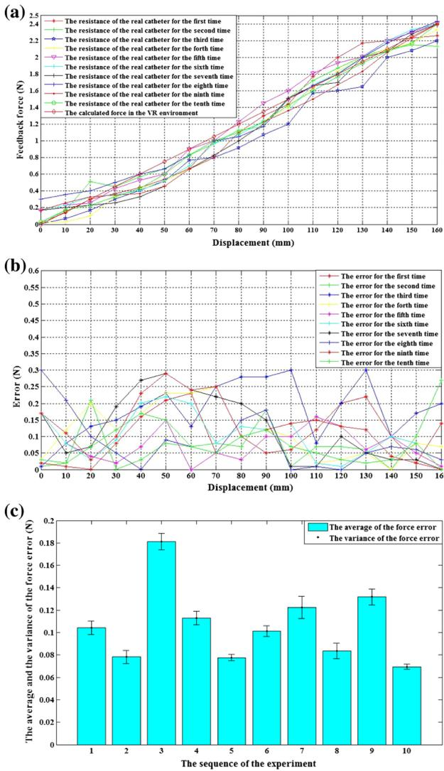
**Fig. 13** The force feedback experiments for ten times. **a** Force feedback experiments for ten times. **b** The error curve of the force feedback experiments. **c** The variance and the average of the force error
