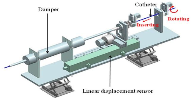
**Fig. 7** Insertion and rotation of the real catheter in master side
