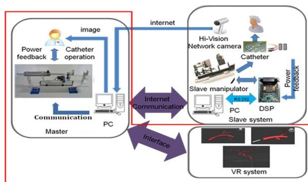
**Fig. 1** The concept diagram for VR- based robotic catheter training system. The master–slave robotic catheter system can realize remote catheter control
