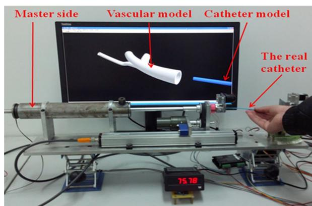
**Fig. 4** The VR-based robotic catheter training system
