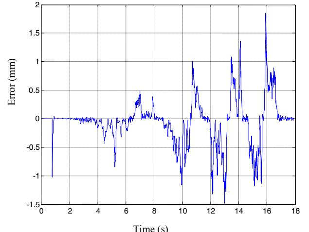
Fig.10 Tracking error of the master-slave system
