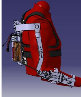
Fig.3 The 3D view of the novel variable stiffness actuator-based exoskeleton for home-based rehabilitation
