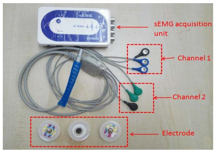
Fig. 2 The sEMG acquisition unit and the electrode
