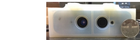
(a) Waterproof cover for the Softkinetic DS525 ToF camera
