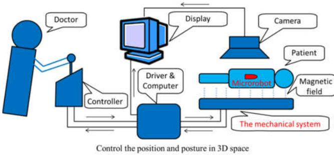
Fig. 1 Electromagnetic actuation system (EMA system)
