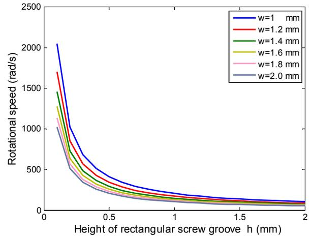
Fig. 7 Simulation results of rotational speed with different parameters of screw groove ( $P=10\text{mN}$  pitch=5mm)
