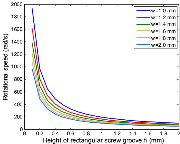
Fig. 6 Simulation results of rotational speed with different parameters of screw groove ( $P=9\text{mN}$  pitch=5mm)
