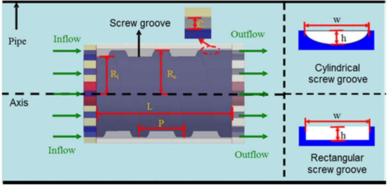
Fig. 4 Propulsive force model
