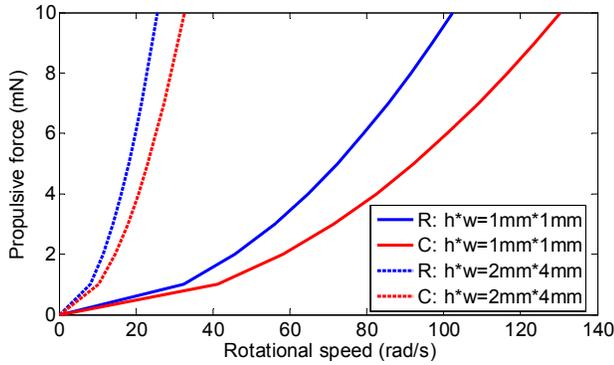
Fig. 5 Compared results with different screw groove, R means rectangular screw groove, C means cylindrical screw groove.
