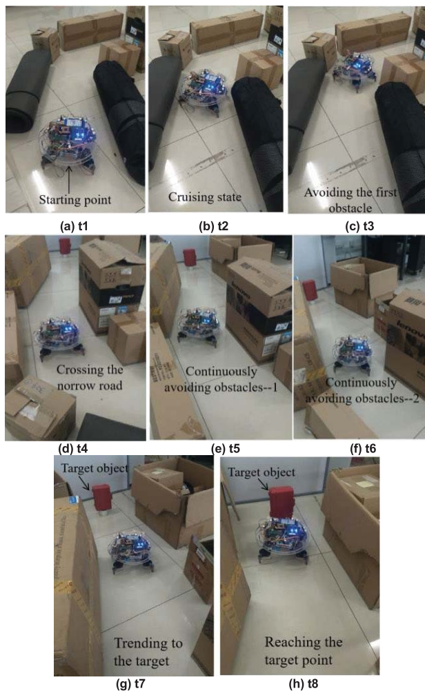
FIGURE 13. Experiments of obstacle avoidance for the spherical robot in complex environment.
