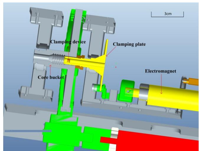
Fig. 5. Partial cross-sectional view of the catheter clamping mechanism in the clamped state.
