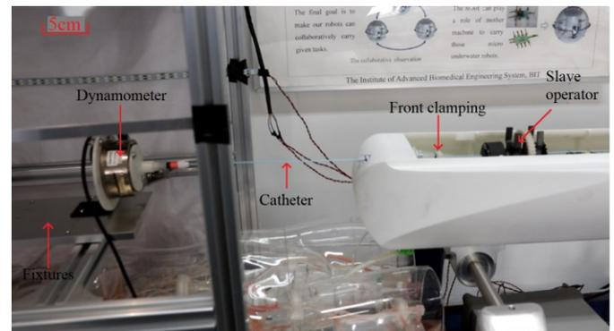
Fig. 6. Actual diagram of the force measuring device.
