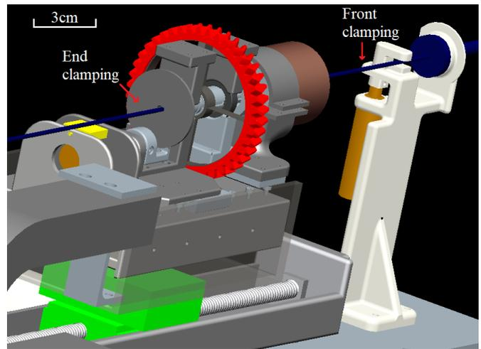
Fig. 4. Conceptual diagram of front clamping and end clamping.
