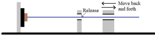
Fig. 8. Friction of the catheter due to movement from the end effector when the end clamp is released.
