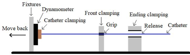
Fig. 7. The friction of the catheter under the clamping condition of the front clamp.
