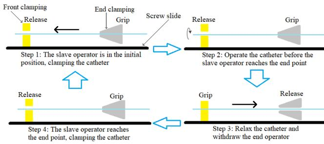
Fig. 2. Schematic diagram of the reciprocating drag operation from the end operator.
