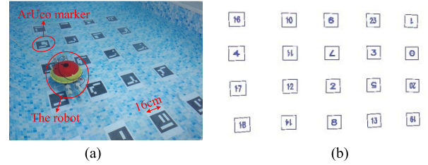
Fig. 16. (a) Experimental setup and (b) the pre-obtained markers array.
