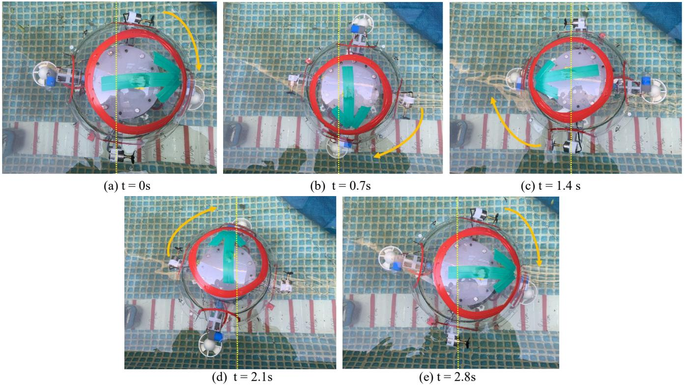
Fig. 7 The rotation-motion progress of the hybrid propulsion spherical underwater robot (HPSUR).
