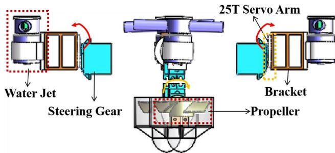
(a) The 3D model of the HPSUR (Slow-steady mode)
