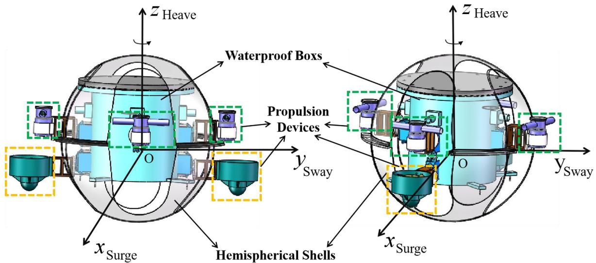
Fig. 1 The overall structure of the hybrid propulsion spherical underwater robot (HPSUR).
