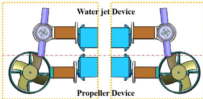
(b) Side view of the hybrid propulsion devices (Fast-flexible mode)
