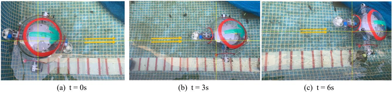
Fig. 5 The forward-motion progress of the hybrid propulsion spherical underwater robot (HPSUR).
