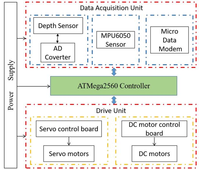
Fig. 4 Control diagram of the HPSUR.
