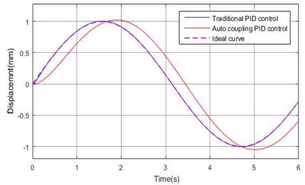
Fig. 8 Sinusoidal response position tracking comparison.
