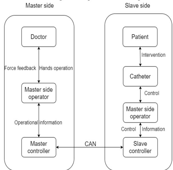
Fig. 1 Control System of Vascular Interventional Surgical Robot.
