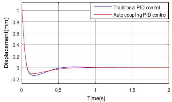
Fig. 9 Step response position tracking error comparison
