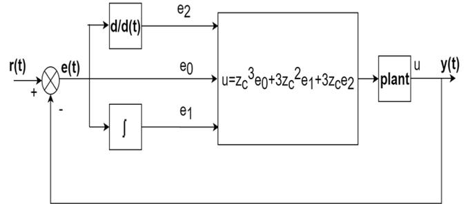
Fig. 5 Autocoupling PID control block diagram
