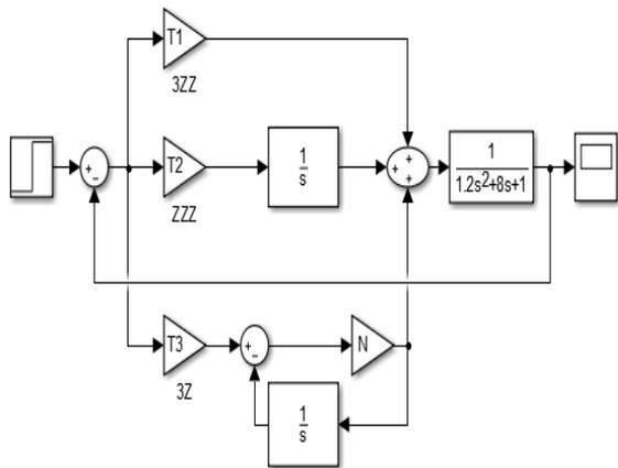
Fig. 6 Block diagram of autocoupling PID logic controller
