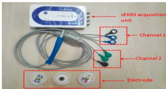
Fig. 2 EMG acquisition equipment
