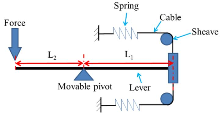
Fig.4. Working principle of the VSA
