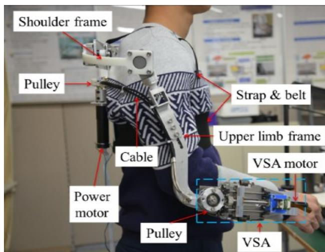
Fig.1. Overall structure design of the PVSED.
