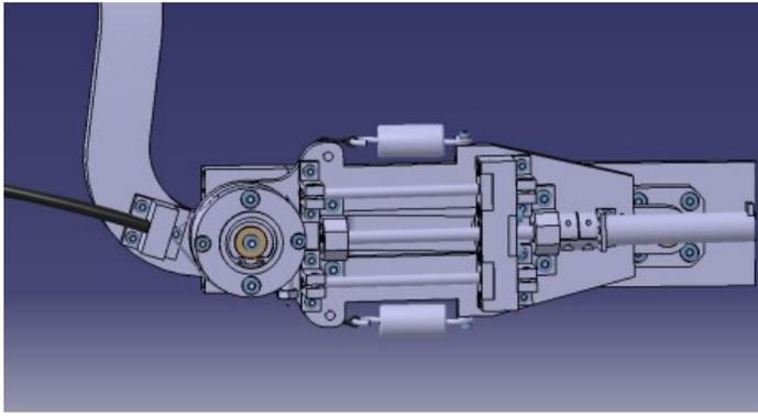
Fig.3. CAD Model of the integrated VSA
