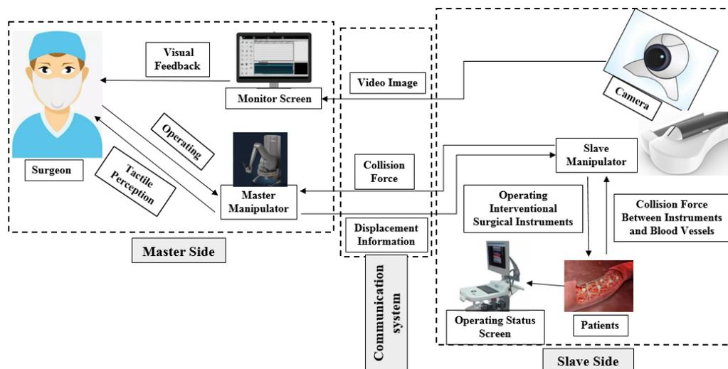
Fig. 1. The master-slave robotic system.
