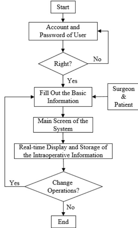
Fig. 6. The workflow of the Intraoperative Information Monitor System.
