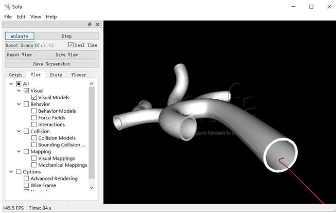
Fig.3 Sofa engine simulation of vascular interventional surgery interface
