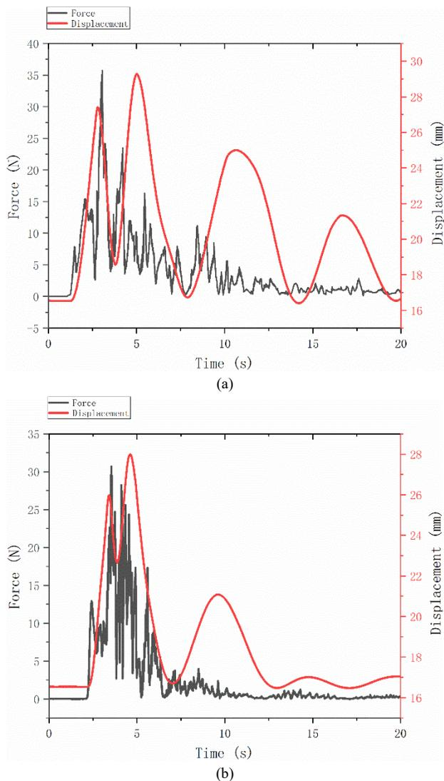
Fig.5 The force and displacement response of the 278th node under the constant force. (a) the displacement and force response of TMM model. (b) the displacement and force response of NVTMM model.
