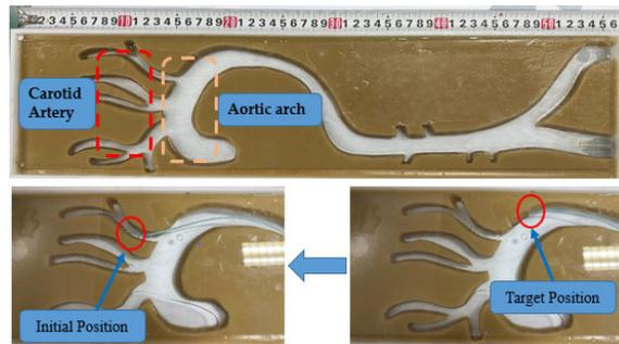
Figure 9. Vascular model in the experiments.
