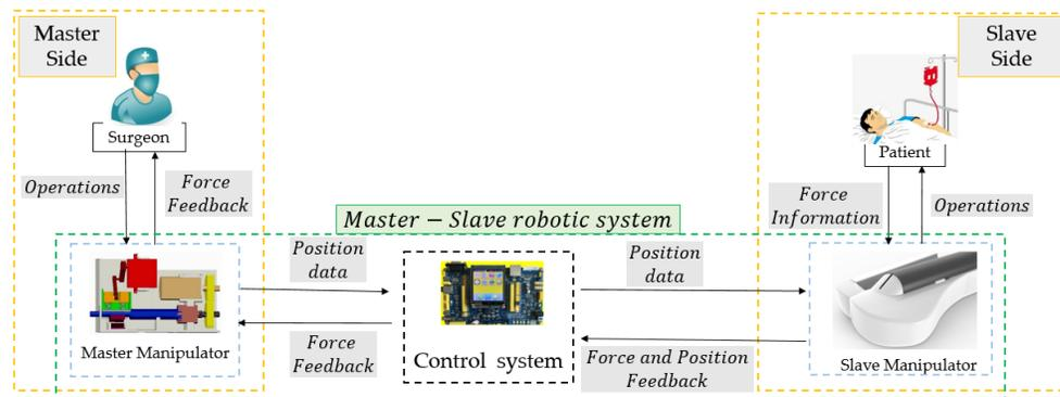
Figure 1. Workflow of the Master–Slave Robotic System.
