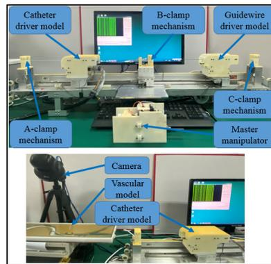
Figure 8. Experimental setup for the evaluation experiments.
