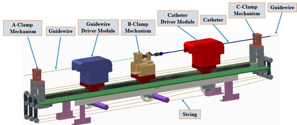
Figure 4. Structure of the slave manipulator.
