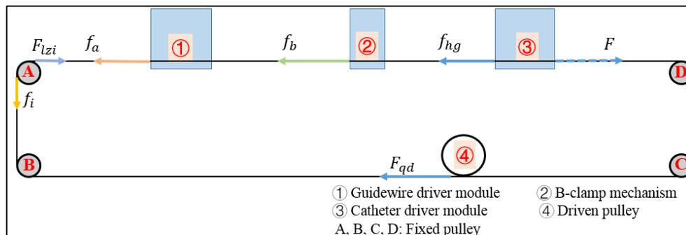
Figure 5. Force analysis diagram of the slave manipulator.
