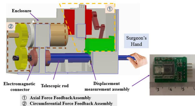
**Figure 3.** Virtual prototype of the master manipulator.
