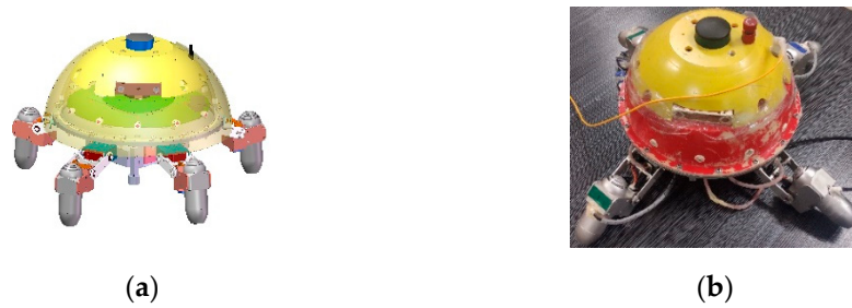
Figure 1. The model structure of the amphibious spherical robot (ASR). (a) The overall appearance of the ASR-V robot; (b) The physical object of the ASR-V robot.
