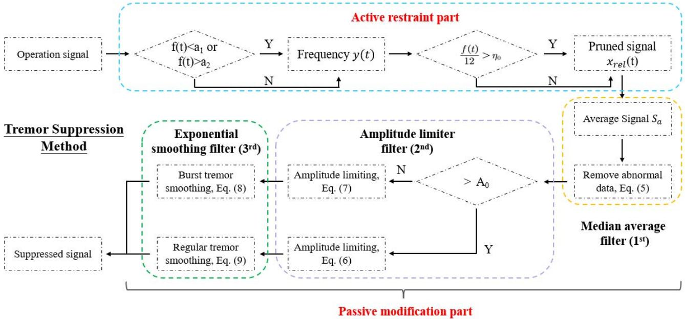
Fig. 7. Flowchart of suppression mechanism for proposed tremor suppression method.
