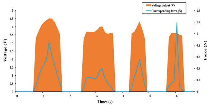
Fig. 10. Voltage output of FSR and corresponding value of force for radial tremor detection.
