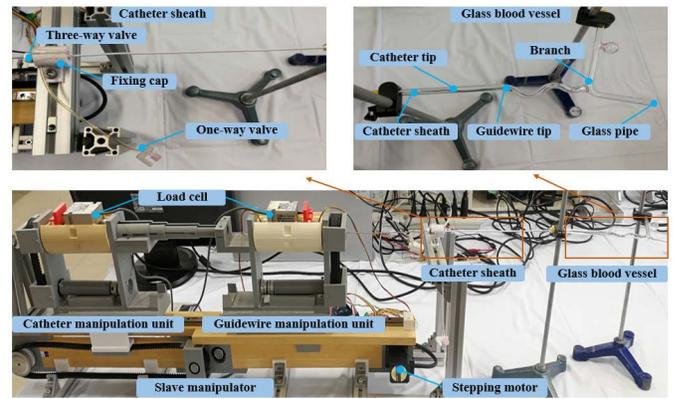
Fig. 12. Experimental setup for glass blood vessel.
