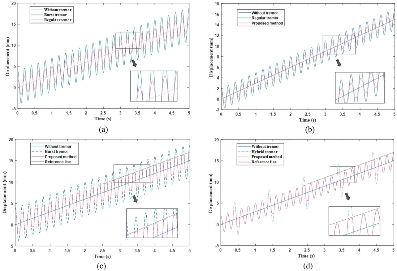
Fig. 9. Results of simulation. (a) Simulation signal without tremor, with burst tremor, and regular tremor. (b) Result for regular tremor with the proposed method. (c) Result for burst tremor with the proposed method. (d) Result for hybrid tremor with the proposed method.
