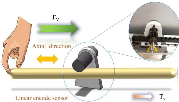
Fig. 5. Force module within axial operation tremor.
