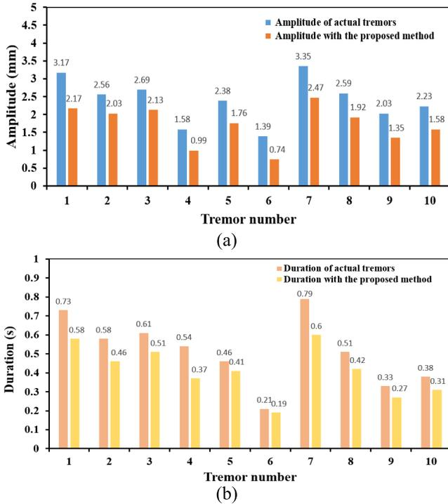
Fig. 15. Comparison qualitative analysis of ten different tremors. (a) Amplitude performance with the proposed method or not. (b) Duration performance with the proposed method or not.
