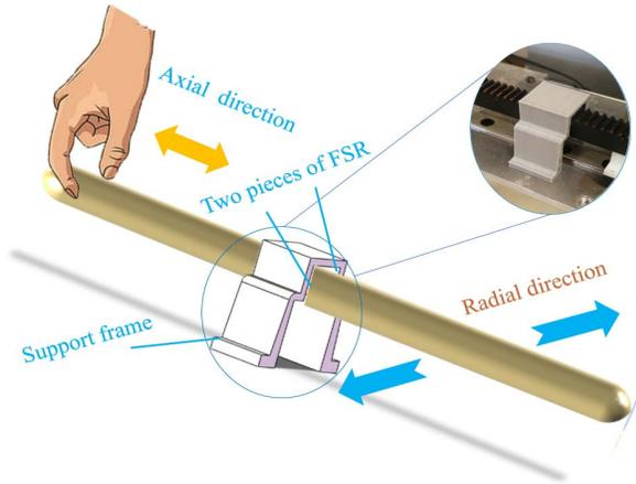
Fig. 4. Radial tremor model of physical form.
