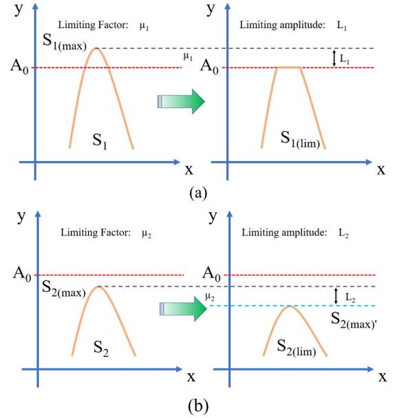
Fig. 6. Mathematical signal models of amplitude limiter filter. (a) Amplitude limiter process for burst/hybrid tremor. (b) Amplitude limiter process for regular tremor.
