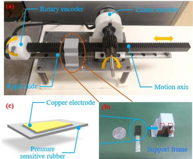
Fig. 3. Self-designed FSR based on pressure sensitive rubber. (a) Actual layout in the master device. (b) Components of the radial tremor detection. (c) Structure of FSR. (Location: The inner walls marked by red boxes.)
