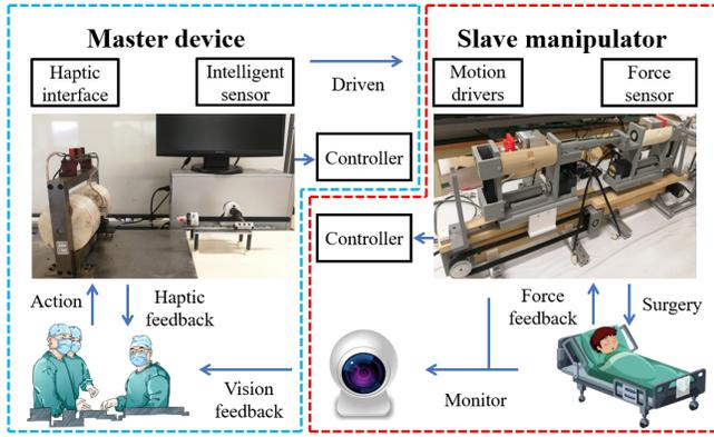
Fig. 2. Conceptual diagram of VIS robot for the robot-assisted surgery.
