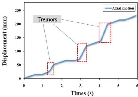
Fig. 11. Tremor detection results for axial encode sensor.
