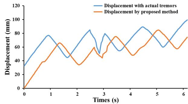
Fig. 13. Comparison displacement results for tremor suppression with the proposed method.
