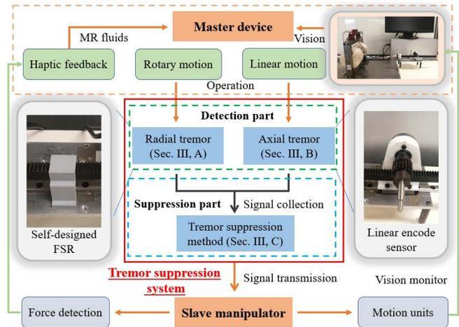
Fig. 8. Framework of proposed tremor suppression system.
