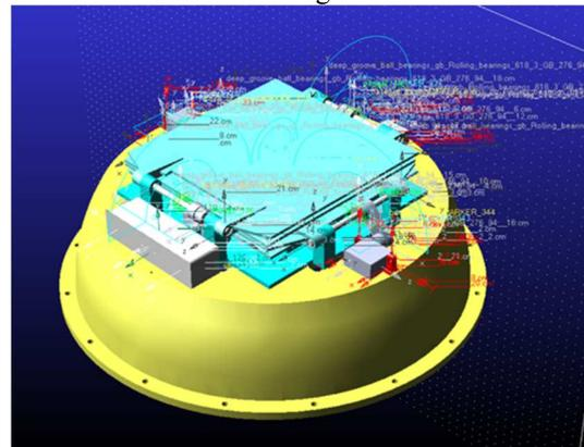
Fig.5. Virtual prototype of the foldable solar harvesting mechanism in the ADAMS platform.
