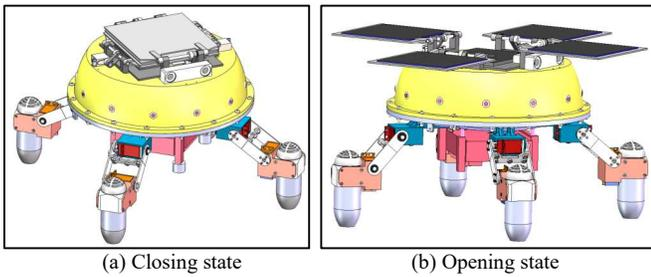
Fig. 3. Opening and closing state of foldable harvesting mechanism.
