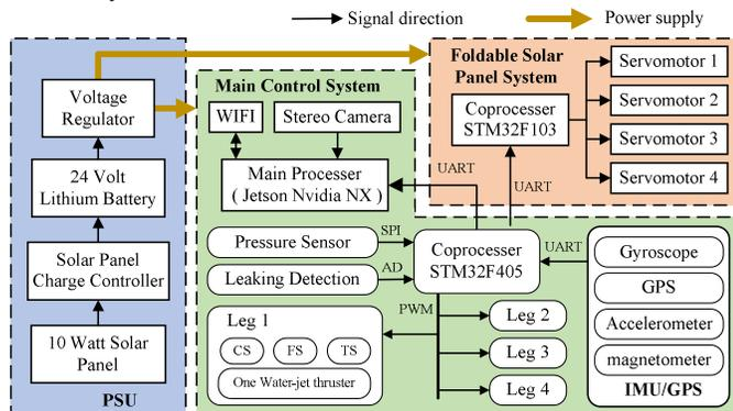
Fig. 4. Electronic control system diagram of the proposed robot.
