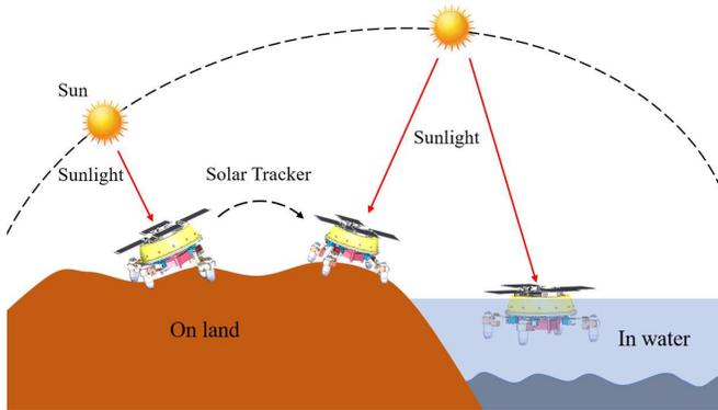
Fig. 1. Schematic diagram of the solar tracker for the amphibious robot. This solar tracker is designed to harvest maximum solar energy in amphibious environments using the foldable solar harvesting mechanism. On land, the robot can adjust the attitude of the solar panels by utilizing four legs. on the surface of the water, the opened solar charging mechanism assists the robot in collecting solar energy.
