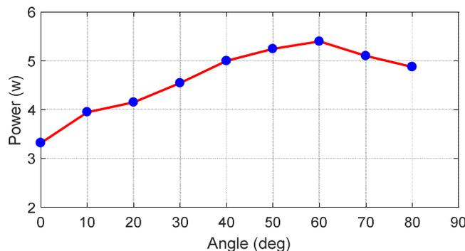
Fig. 10. The output power of solar panels at different attitudes.
