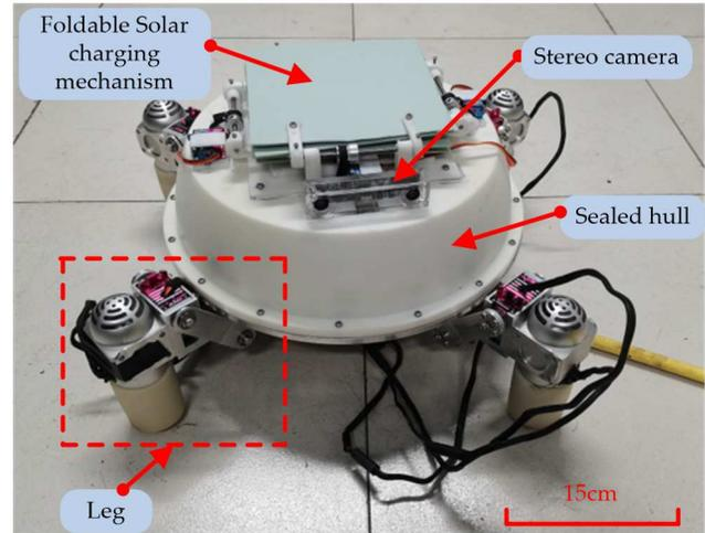
Fig. 2. The overview structure of the developed amphibious robot.
