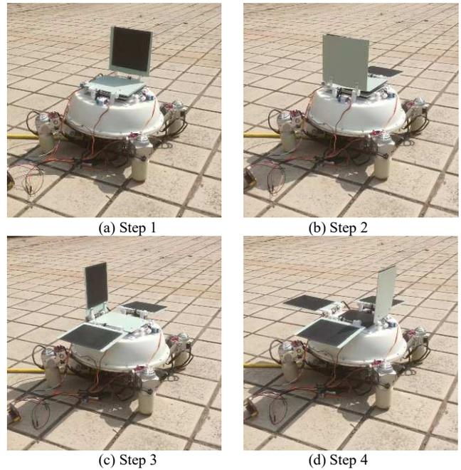
Fig. 8. Open and close control of the foldable mechanism.
