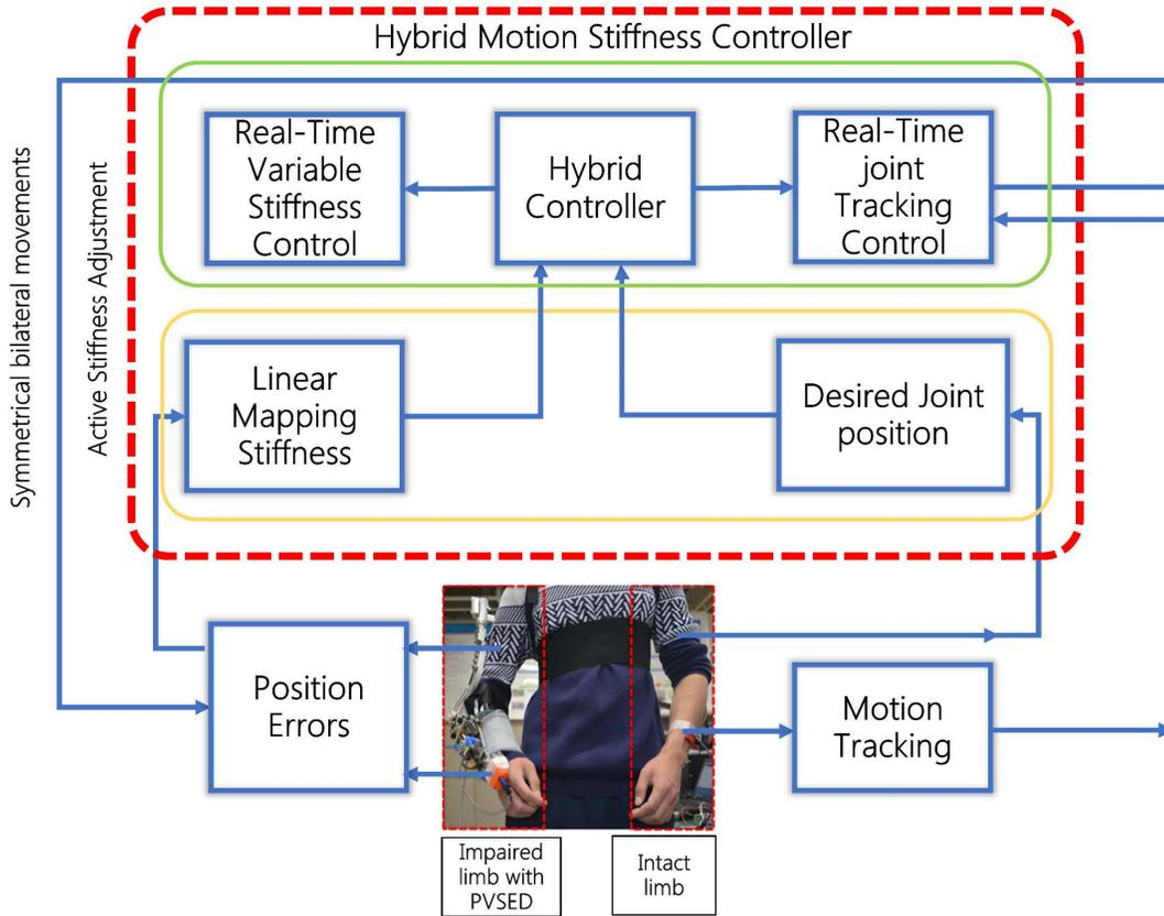
Fig. 4. The Control diagram of the proposed hybrid motion stiffness control.
