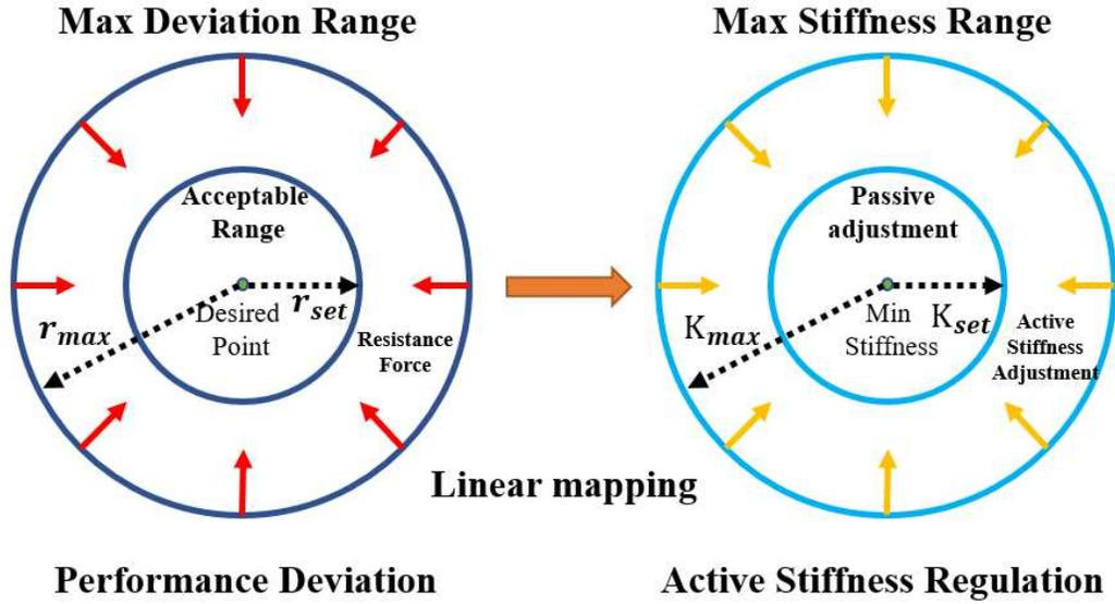
Fig. 5. The linear mapping from the position errors to robotic stiffness.
