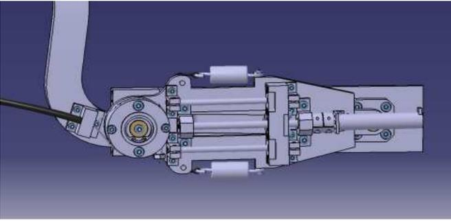
Fig. 2. The CAD mechanical design of the PVSED.
