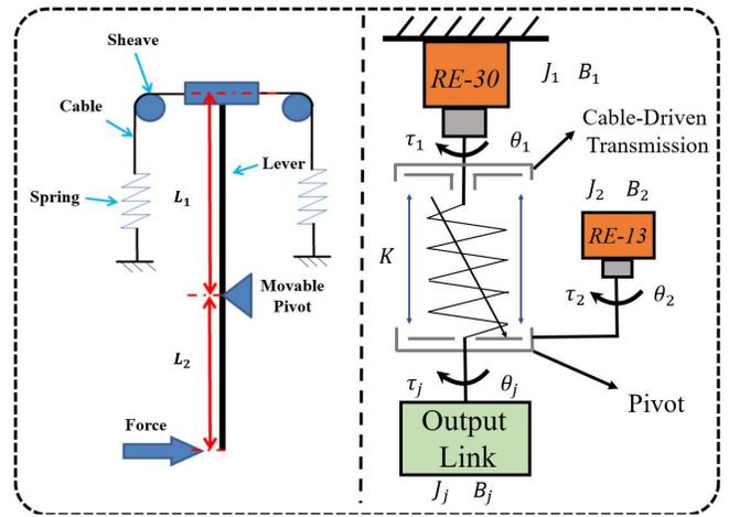
Fig. 3. The working principle of the VSA
