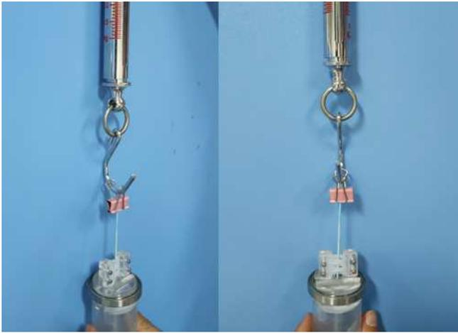
Fig. 7. Measure the maximum push force.
