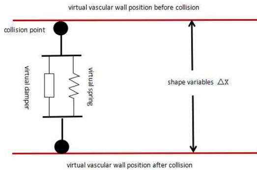
Fig.3 Collision force model
