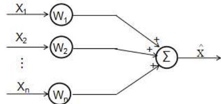
Fig.7 Schematic diagram of weighted fusion algorithm
