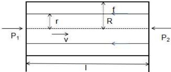
Fig.6 Viscous resistance schematic
