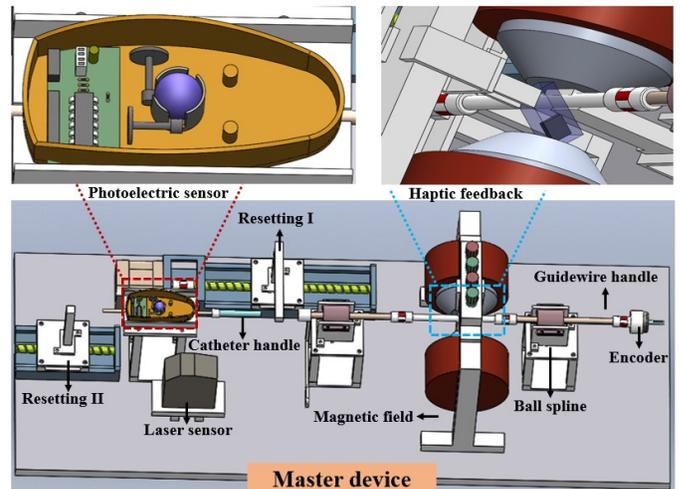
Fig. 2 The master device based on collective operating handles.
