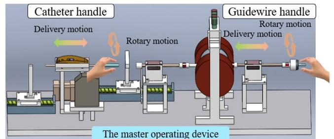
Fig. 4 The installation view and achieving mechanism of haptic feedback.
