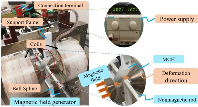
Fig. 3 The installation view and achieving mechanism of haptic feedback.
