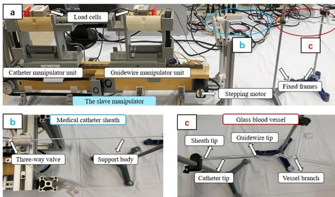
Fig. 5 The experimental setup for performance evaluation. (a) The slaver manipulator. (b) Medical catheter sheath. (c) Glass blood vessel.
