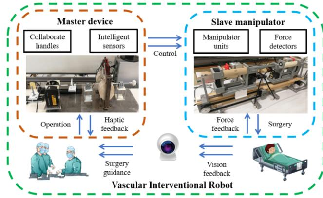
Fig. 1 Conceptual diagram of the developed vascular interventional robot.
