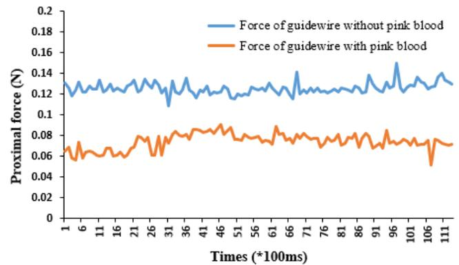
Fig. 7 Comparative results of proximal force for guidewire
