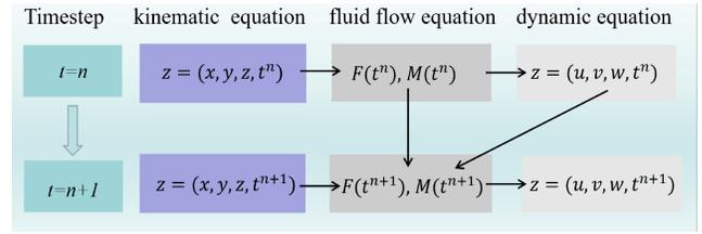
Fig. 4. The sketch of the coupling equation and its solution
