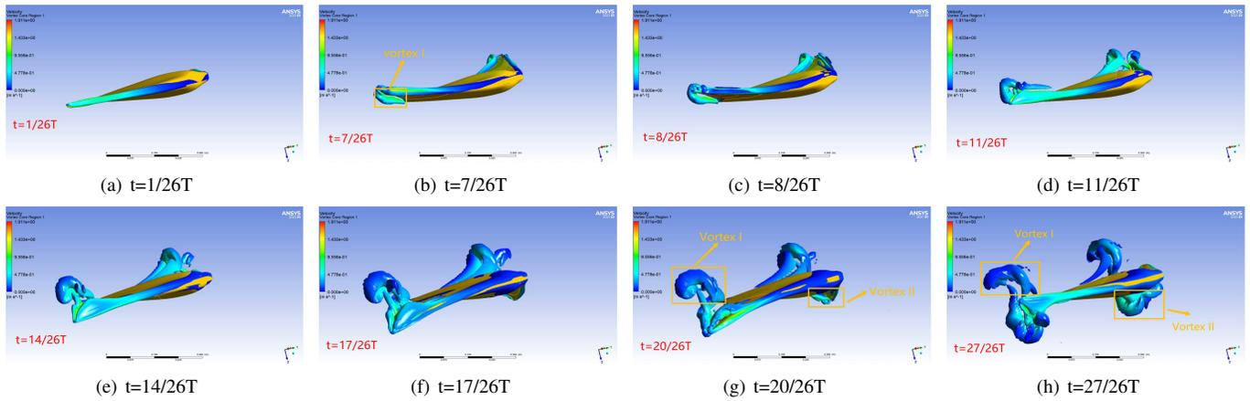
Fig. 6. Vortex structure during the first self-propelled cycle
