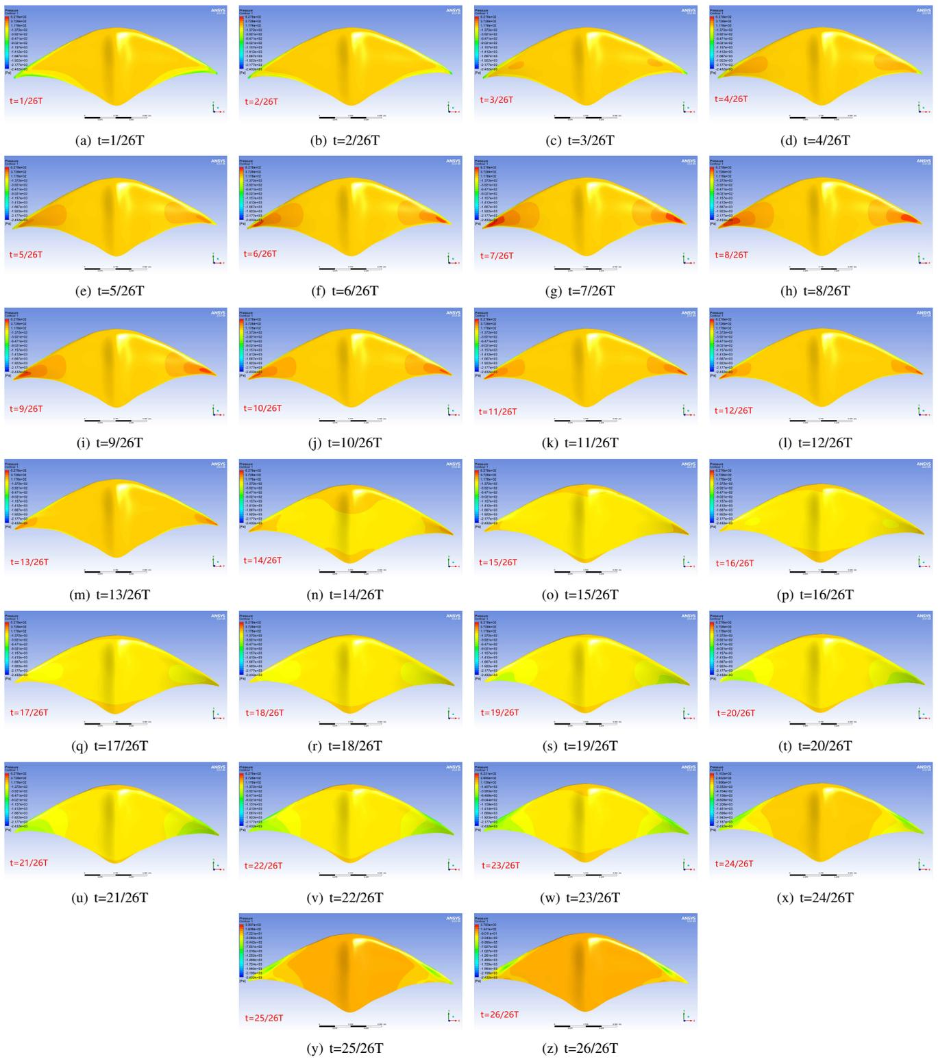
Fig. 5. Pressure contour during one self-propelled cycle
