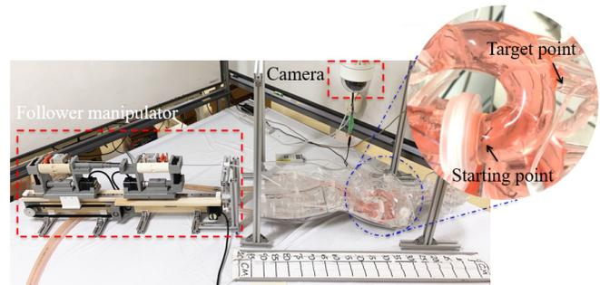
Fig. 13. Experimental setup in EVE model (pressure: 120/80 mmHg).
