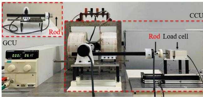
Fig. 3. Structure of the MR fluids-based leader manipulator (GCU has not yet incorporated haptic feedback, and CCU has incorporated haptic feedback).
