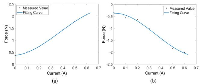
Fig. 5. Relation between the haptic force generated by the MR fluids and the electric current. (a) Tension. (b) Thrust.
