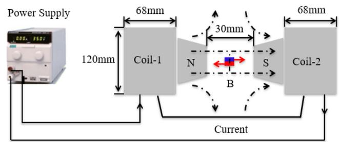
Fig. 4. Method of providing the external magnetic field.
