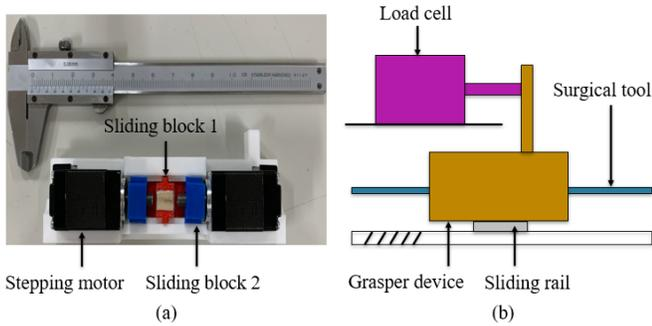
Fig. 7. Grasper device and the force sensing method. (a) Grasper device. (b) Proposed force sensing method of the flexible instrument.
