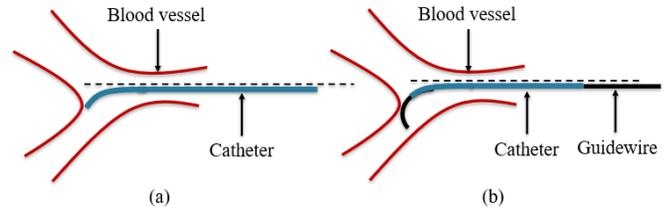
Fig. 8. Concept of two operating methods. (a) Method of only operating the catheter. (b) Concept of the collaborative operation of the guidewire and the catheter.
