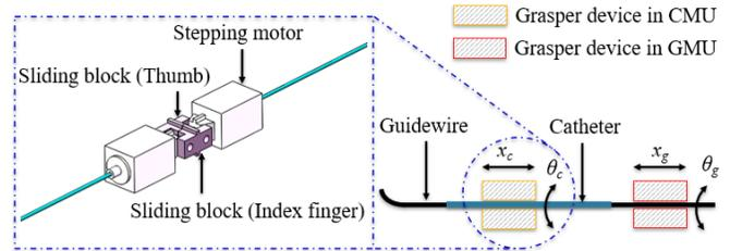
Fig. 9. Operation process of using two grasper devices to perform the delivery of the guidewire and the catheter.
