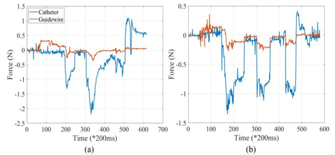
Fig. 14. Real-time force of the flexible instrument during the operation. (a) Without haptic feedback. (b) With haptic feedback.
