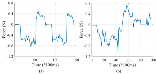
Fig. 12. Real-time force of the flexible instrument during the operation. (a) Failed sample. (b) Successful sample.
