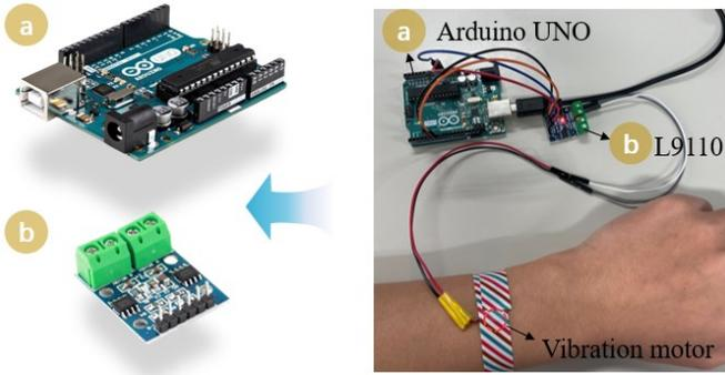
Fig. 6 Experiment setup for loudness and sensing. (a) Arduino UNO; (b) L9110 driven module.
