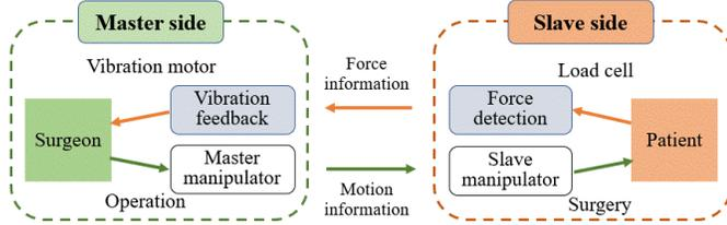
Fig. 5 The transfer model of vibration feedback for the robotic system.
