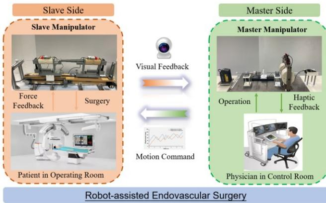
Fig. 1 Conceptual diagram of the robot-assisted endovascular surgery.
