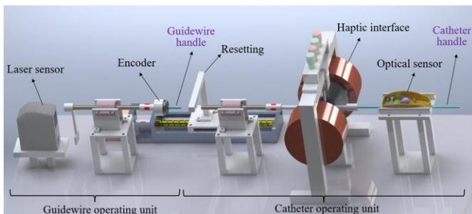
Fig. 2 The developed master manipulator for RES system.
