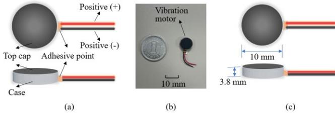
Fig. 4 The details of vibration motor. (a) elaborate components; (b) real layout; (c) dimension parameters. (Top view and main view)
