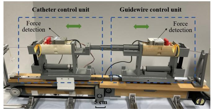
Fig. 3 The slave manipulator based on collective operating handles.
