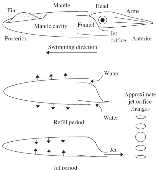
**Fig. 8** Sketch of the structures and propulsive mechanisms of the long-finned squid [73]
