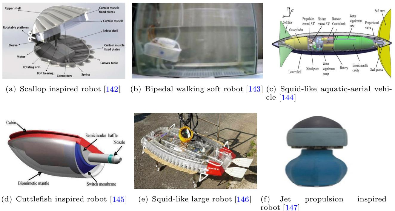
**Fig. 15** Jet-based inspired robot, where **a**, **c**, **d**, **e** and **f** use jet to propel and **b** simulate the walking with octopus feet. Specifically, the **c** is a small robot and **e** is a large robot and others are common sized
