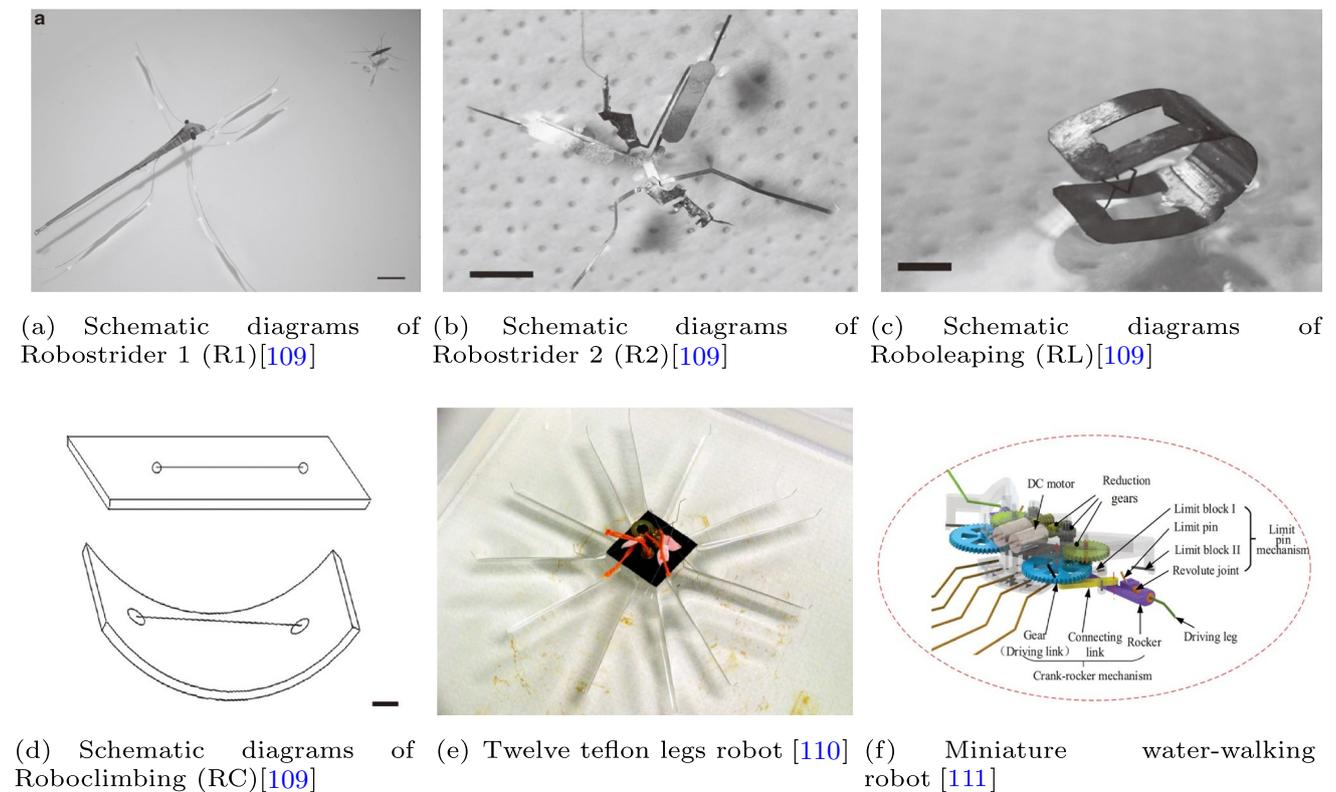
**Fig. 11** Interface-based inspired robot, where **b, c**, are micro-sized and **a, d, e** and **f** are small-sized robot. The prototype of the above robots is water striders and other aquatic insects
