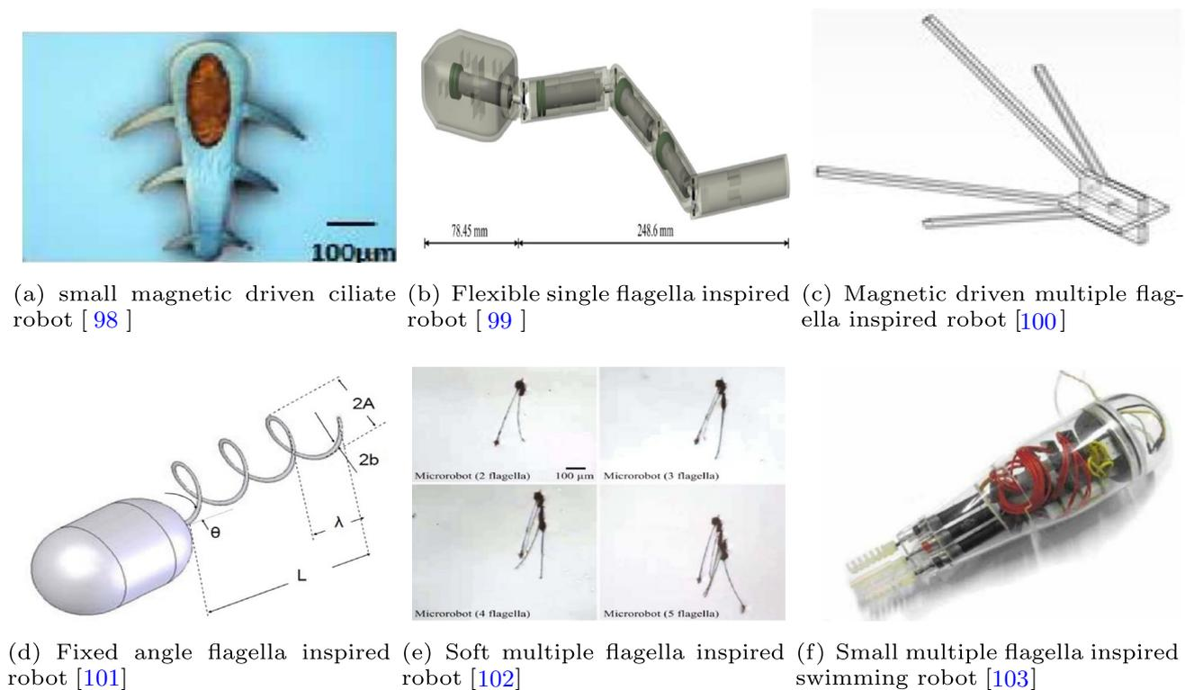
**Fig. 10** Drag-based inspired robot. The prototype of the above robots are ciliates and flagellates
