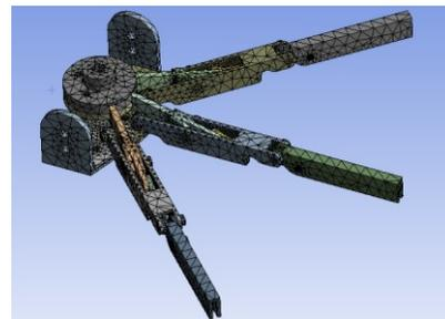
Fig. 11. Three dimensional elastoplastic finite element model of optimized webbed feet
